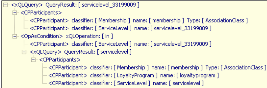
Figure 5.2 AST of IN operation
