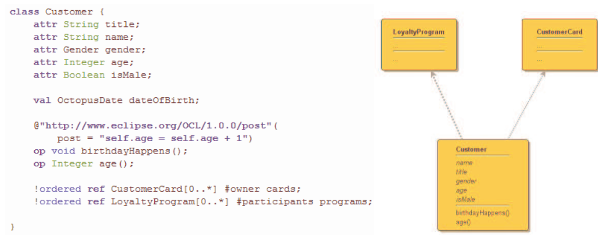
Figure 3.5: An EReference presents in Emfatic editor and the representation of it in EMF diagram.
