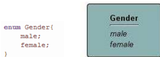
Figure 3.3: An EEnum presents in Emfatic editor and the representation of it in EMF diagram.
