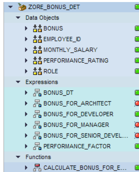
Fig. 6.15: Data Objects, Expressions and Functions in BRFplus with activation status
