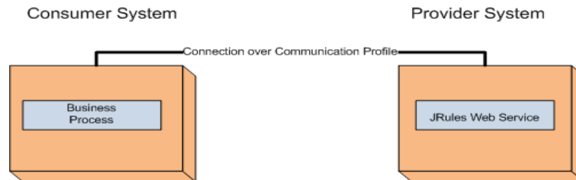
Fig.7.1.: JRules Web Service is hosted on a Provider System and is accessed through a Communication Profile
