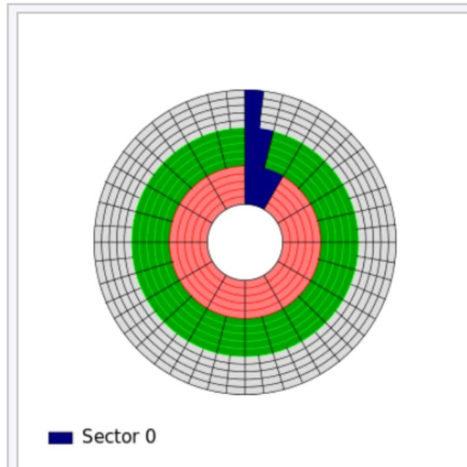
Physical layout of sectors in a zone-bit disc: As distance from the centre increases, the number of sectors in a given angle increases from one (red) to two (green) to four (grey).
